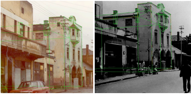
Figure 9: Perceptual test of the British Bioscope reconstruction. Edges in the reconstructed geometry (in green) are overlaid onto the original photograph and closely conform to user drawn edges (still partly visible in red).
