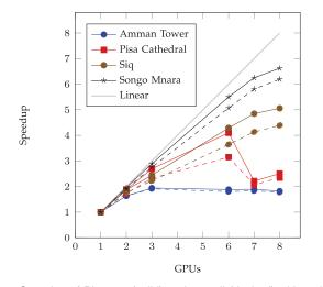
Fig. 13. Speedup of Phase 2 (solid) and overall (dashed) with multiple GPUs. For up to three GPUs, a single node is used. The remaining data points use two, three, and four nodes, respectively. There are two 3-GPU and two 1-GPU nodes.
