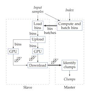
Fig. 10. Phase 2 data flow in a cluster. Each dotted box represents one node in the cluster and the double arrows show data passed by MPI messages. Only one of the slaves is shown. The master may also act as a slave if it has GPUs. Color-coding is as for Fig. 2.
