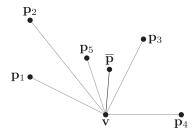
Fig. 7. Boundary detection. Given a point  ${\bf v}$  on the MLS surface, the neighborhood  ${\bf p}_i$  is used to compute a weighted mean  $\overline{\bf p}$ . If  ${\bf v}$  lies outside the boundary, the neighborhood will be skewed to one side of  ${\bf v}$  and so  $\overline{\bf p}$  will be far from  ${\bf v}$ .
