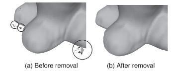
Fig. 8. Removal of isolated components.
