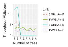
**Fig. 8.** TVWS and 5 GHz WiFi throughput through trees.
