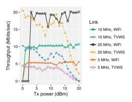
Fig. 6. Throughput vs txpower.
