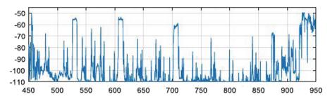
(a) TVWS band spectrum scan. Vertical axis: uncalibrated signal strength; horizontal axis: frequency in MHz.
