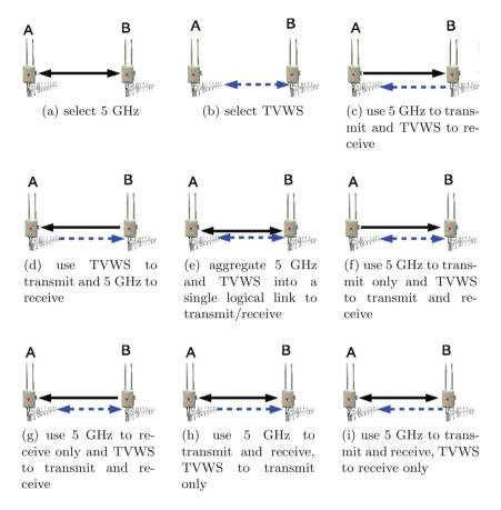
**Fig. 3.** Possible options when using 5 GHz and UHF-TVWS hybrid links. The black solid line and blue dashed line respectively represent 5 GHz and UHF-TVWS radio links. (Color figure online)
