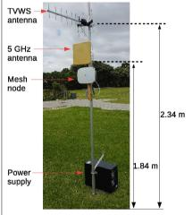
Fig. 5. Node specifications and physical setup.
