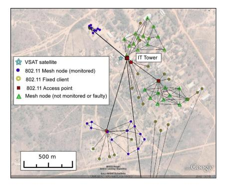
*Figure 2. View of the Macha network. Network traffic is monitored at the satellite link gateway.*
