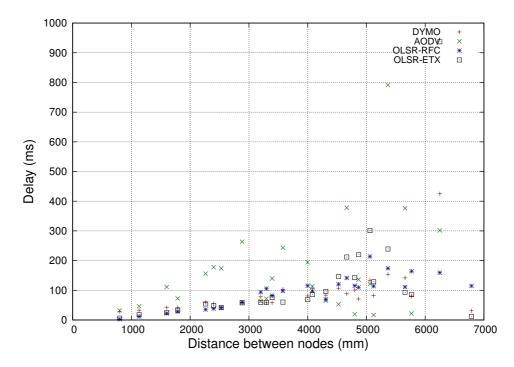
Figure D.7: Avrage round trip delay vs distance for ping tests between nodes in 7x7 grid.
