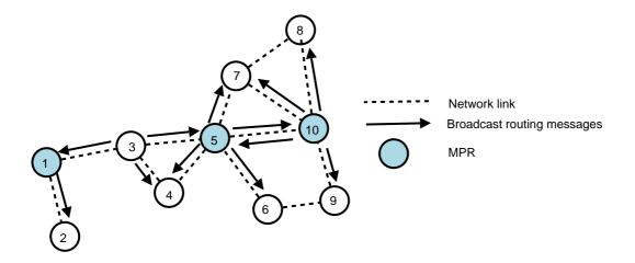
Figure 2.4: OLSR routing protocol showing selection of MPRs.
