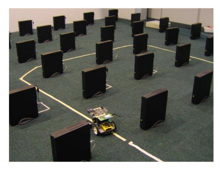
Figure 3.1: Layout of the 7x7 grid of Wi-Fi enabled computers. The optional line-following robot will be explored in the future to test mobility in a mesh network.
