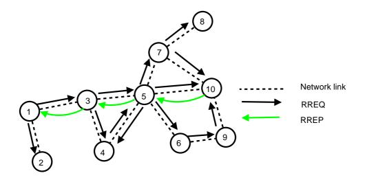
Figure 2.2: AODV routing protocol showing the route discovery process.
