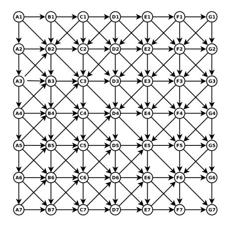
Figure 4.10: All possible connections between nodes if signal radius is greater than or equal to  $\sqrt{2}$  and less than 2 in a unit-spaced grid and all vertices in a path decrease the distance to the destination.
