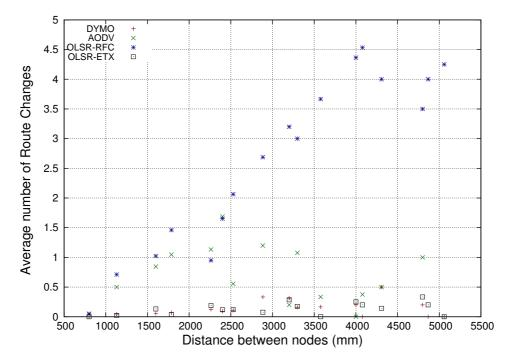
Figure C.6: Avrage number of route change vs distance for ping tests between nodes in 3x7 grid
