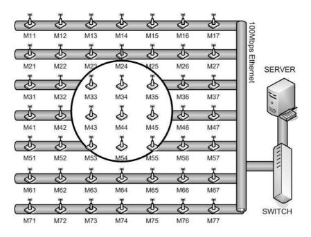
Figure 3.3: The architecture of the mesh lab. Ethernet is used as a back channel to connect all the nodes to a central server through a switch. Each node is also equipped with an 802.11 network interface card.
