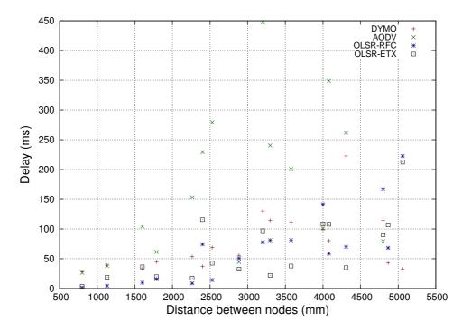
Figure C.7: Avrage round trip delay vs distance for ping tests between nodes in 3x7 grid.
