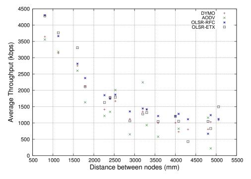
Figure C.4: Average throughput vs distance in 3x7 grid.
