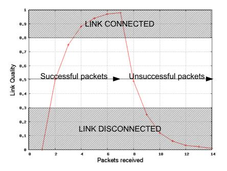
Figure 2.5: Link Hysteresis in the OLSR routing protocol.
