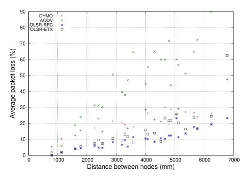
Figure D.5: Average packet loss vs distance for ping tests between nodes in 7x7 grid.
