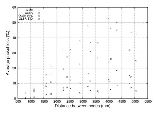
Figure C.5: Average packet loss vs distance for ping tests between nodes in 3x7 grid.
