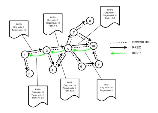
Figure 2.7: DYMO route discovery process showing how path accumulation is used to discover a route from node 1 to node 10.
