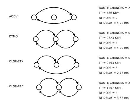
Figure 5.3: Topology created by each MANET routing protocol for a simple string of pearls 3 nodes long.
