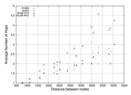
Figure C.3: Average hop count vs distance for ping tests between nodes in 3x7 grid.
