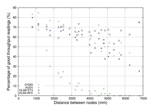
Figure D.2: Percentage of good readings vs distance for throughput tests between nodes in 7x7 grid.
