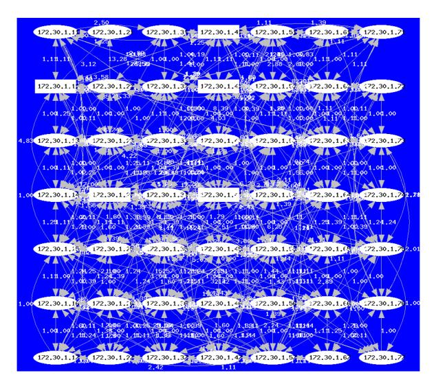
Figure 5.2: OLSR topology using the ETX metric showing good multi-hop characteristics. The wireless NICs were configured to 802.11b mode, 11 Mbps data rate and power level set to 0 dBm.
