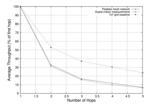
Figure 6.5: Comparison of theoretical, indoor and outdoor throughput.
