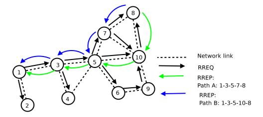
Figure 2.3: *Route discovery process for DSR showing how a route is discovered from node 1 to node 8. Only optimal routes are shown to simplify the diagram.*
