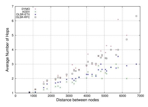
Figure D.3: Average hop count vs distance for ping tests between nodes in 7x7 grid.
