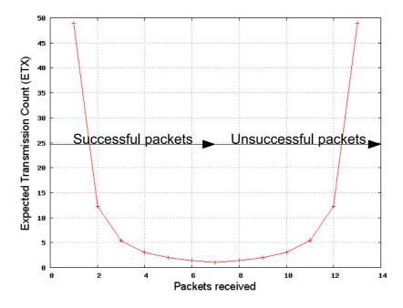
Figure 2.6: ETX path metric values for successive successful and unsuccessful packets.
