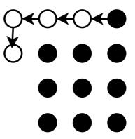
Figure 3.5: Growing spiral topology for tests which compares a metric against a growing network size.
