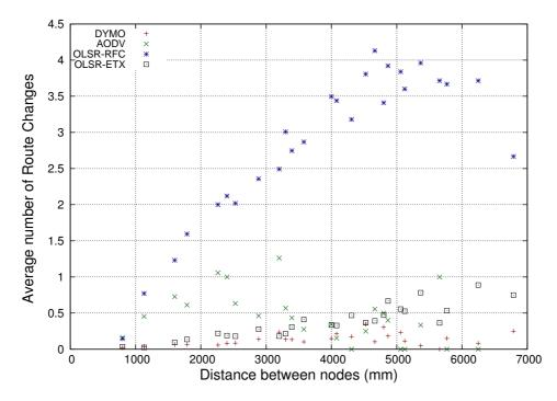
Figure D.6: Avrage number of route change vs distance for ping tests between nodes in 7x7 grid
