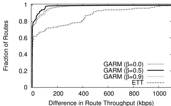
Fig. 2. Accuracy of gateway selection: CDF of difference in throughput using the GARM and ETT routing metrics compared to that using the Oracle approach (best gateway). A perfect routing metric has zero difference.
