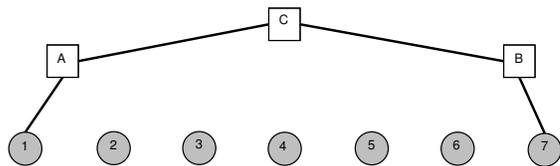
Fig. 1. Simple Line Topology: The gray circles are mesh nodes. Gateway nodes 1 and 7 are connected to routers A and B via Ethernet-like connections. We measure the throughput to node 5.
