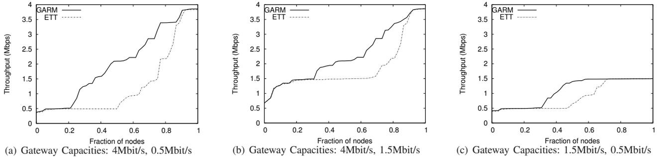
Fig. 3. Distribution of node TCP throughput with different gateway capacities. GARM increases throughput for up to 67% of the nodes. The performance increases as the the difference in gateway capacities grows.
