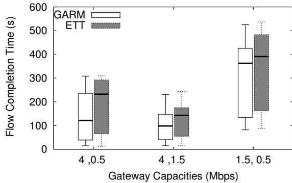
Fig. 4. Distribution of time required to download a 5 MByte file in the UCSB MeshNet.
