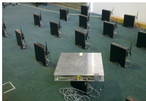
Figure 4. Picture showing the position of the antenna on the node and an overview of the wireless mesh network laboratory.
