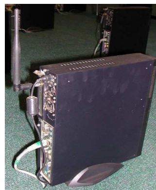
Figure 5. A closer look at an individual node: the RS232 connector is just above and next to the white/green Ethernet cable. The antenna is connected to the wireless card via a 30 dB attenuator.
