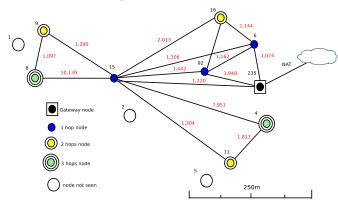
Figure 5: Scaled snapshot of the miam mesh during the 2 week measurement period with ETX values indicated per link. Note that the number hops is determined by the route with the lowest sum of ETX values.
