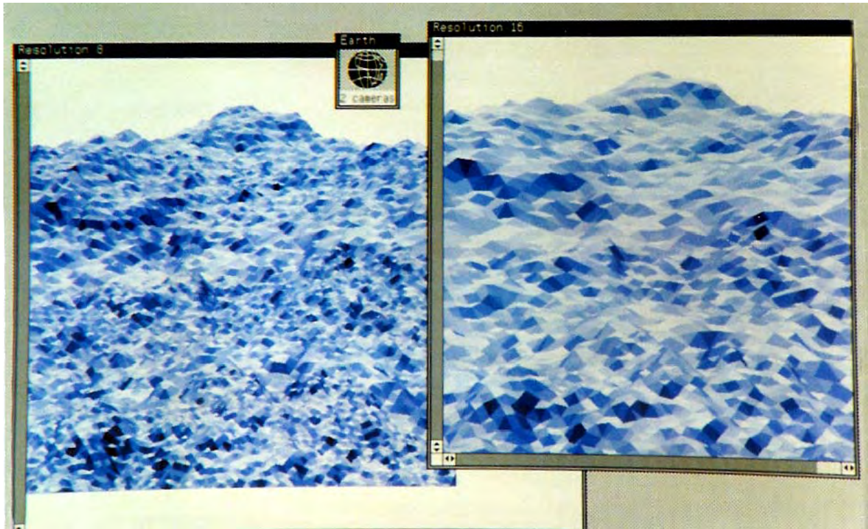
Figure 6.8. Fractal mountain viewed by two cameras at different resolutions. The nominal facet sizes in pixels are given in the frame labels (8 & 16). The same facet size was maintained in spite of increasing distance; both in the given (Fourier synthesized) landscape and in the generated parts. This same method was used in Figure 6.7, but at the higher resolution, as intended, the mechanism cannot be seen.
