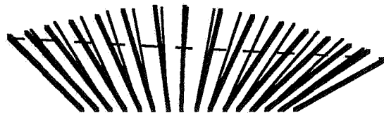
Figure 1. The different rates for linear and angular interpolation.
