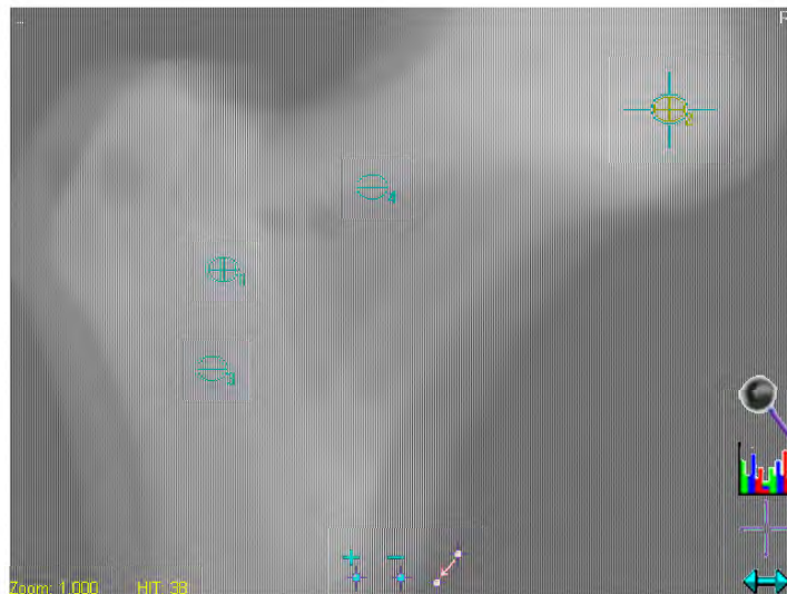
Figure 53: A screen shot of the X-ray viewer application. The viewer is running in column interlaced stereo mode. This is an alternative to the page flipped stereo format supported by WINx3D. This stereo format is not supported by the Nvidia based graphics cards.
