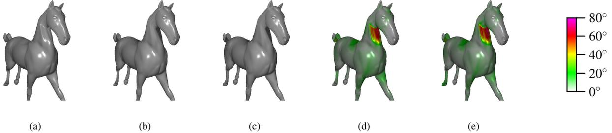
Figure 1: Normal transformation methods and their angle errors. (a) Correct transformation (equation (1)). (b), (c) Equations (2), (3) — note the lack of highlights on the neck and displaced highlights on the body. (d), (e) Errors introduced by equations (2), (3).
