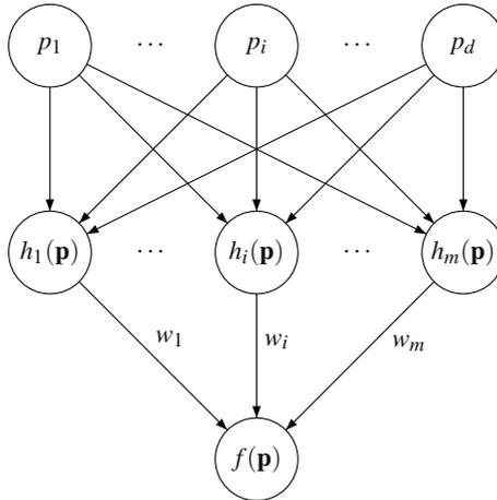
**Fig. 2** A traditional RBFN accepts input from an  $d$ -dimensional vector,  $\mathbf{p}$ , which is fed forward to the  $m$  hidden units  $h_i$  ( $i \in 1 \dots m$ ). The outputs from the hidden units are then each weighted by  $w_i$  and summed to give the result,  $f(\mathbf{p})$ .
