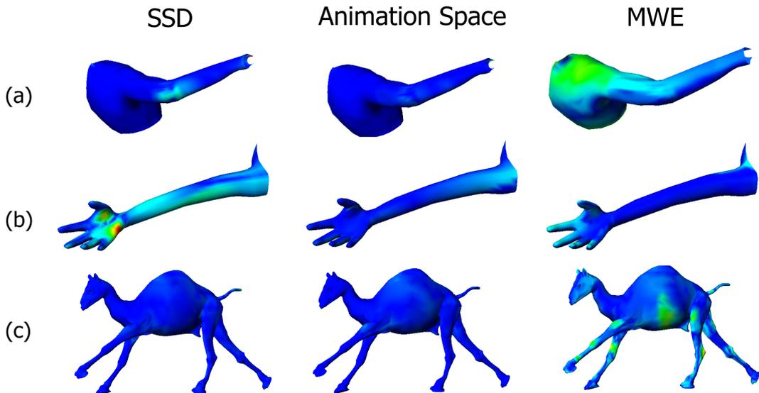
**Figure 4:** *The geometric deviation for the armposes (a), twist (b) and camel (c) data sets. A training set of size 4, 3 and 6 respectively was used to train the skinning frameworks. The SSD arm and twist exhibit joint collapse and candy-wrapper defects while MWE shows signs of over-fitting.*
