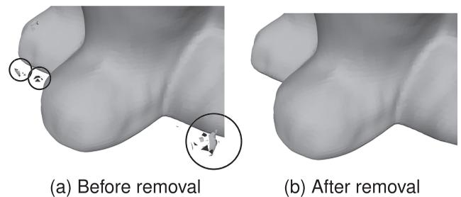
Fig. 8. Removal of isolated components.
