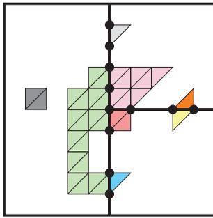
Fig. 9. Identifying components. The thick lines delineate bins, and each clump is given a different color. The external vertices are marked with dots. Note that global information is required to correctly identify small components for deletion: The blue clump (bottom) contains only one triangle, but is a part of the largest global component.
