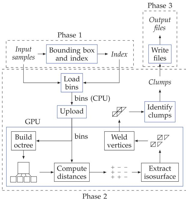
Fig. 2. Data flow in the system. The blue boxes represent independent threads connected by queues, while italics indicate data on disk.
