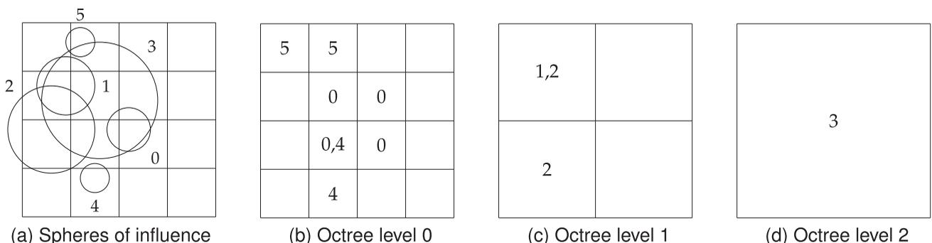
Fig. 3. Example 2D analogue of an octree. Levels are shown fine-to-coarse from left to right. Numbers in the nodes are the IDs of samples that should be considered when visiting the node.
