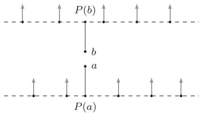
Fig. 5. Misalignment of scans causes a discontinuity in the signed distance. The dashed lines represent the two different scans of the same surface, which have been misaligned. Query points  $a$  and  $b$  are close, but  $a$  projects onto the lower sheet and is considered outside, while  $b$  projects onto the upper sheet and is considered inside. Isosurface extraction infers a spurious isovortex between  $a$  and  $b$ .
