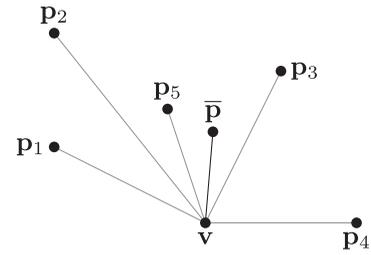
Fig. 7. Boundary detection. Given a point  $v$  on the MLS surface, the neighborhood  $p_i$  is used to compute a weighted mean  $\bar{p}$ . If  $v$  lies outside the boundary, the neighborhood will be skewed to one side of  $v$  and so  $\bar{p}$  will be far from  $v$ .
