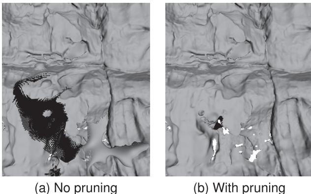
Fig. 6. Without boundary pruning there are significant artifacts. Boundary pruning eliminates the artifacts, although it also opens up some holes that were otherwise filled.
