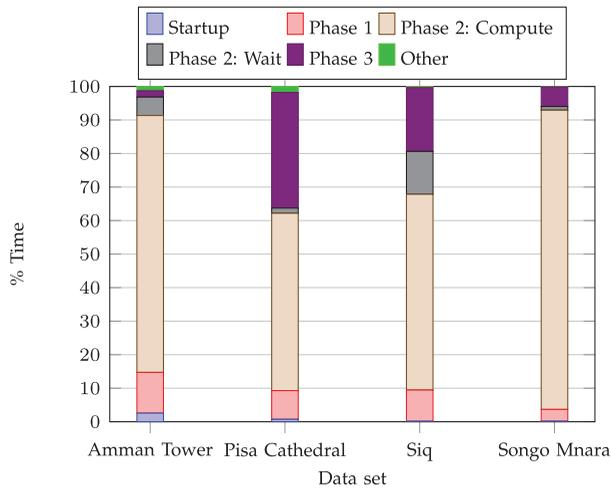
Fig. 12. Time breakdown. Phase 2 is subdivided into time spent in the GPU thread (“Compute”) and time spent waiting either for more input to arrive or for more space in the output buffer (“Wait”). “Other” is time not accounted for in any of the phases, particularly freeing of resources.
