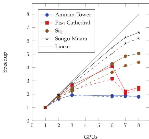
Fig. 13. Speedup of Phase 2 (solid) and overall (dashed) with multiple GPUs. For up to three GPUs, a single node is used. The remaining data points use two, three, and four nodes, respectively. There are two 3-GPU and two 1-GPU nodes.
