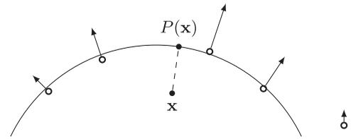
Fig. 1. Projection operation for APSS. The hollow circles represent splats, with arrows representing normal direction and arrow length representing the weight  $w_i(\mathbf{x})$ . The initial point  $\mathbf{x}$  is projected onto the fitted sphere to give  $P(\mathbf{x})$ .
