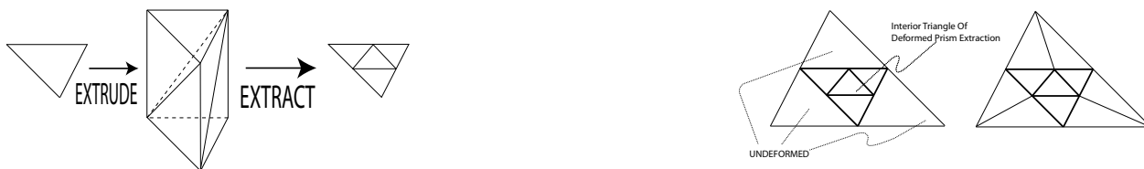
Figure 4: [Left] A triangle is extruded to define a prism which is subdivided into tetrahedra. The undeformed subdivided prism will produce four triangles filling the original shape. [Right] when deformed and undeformed triangles are neighbours, a two-manifold mesh is produced by connecting the new vertex to the apex of the undeformed triangle.
